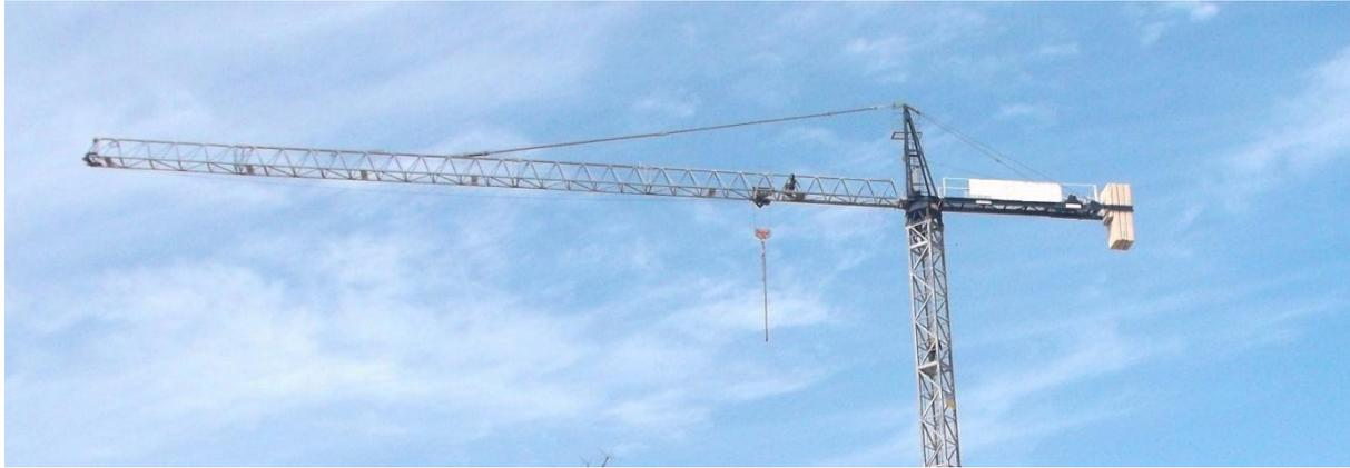
4. Tower cranes should only be erected on gradients within limits specified by the manufacturer. Tower cranes should only be erected at a safe distance from power lines, excavations and ditches as recommended by the competent person.
